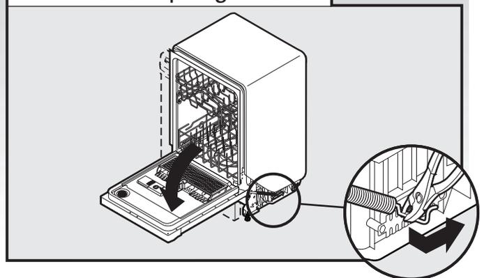
If the door falls open, increase the spring tension by moving the spring end toward the back of the dishwasher.
